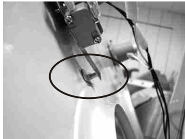
3. Fix the screw to start the snap-lock wire connector.
